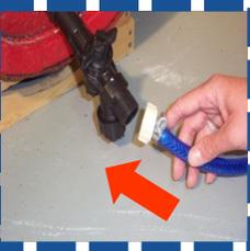
Reconnect coupling with filter washer
