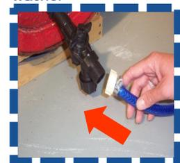
Reconnect coupling with filter washer
