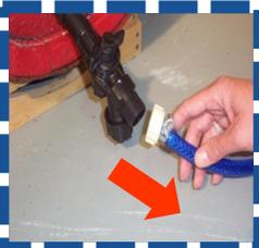
Remove coupling and any filter washer
