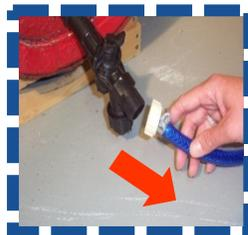
Remove coupling and any filter washer
