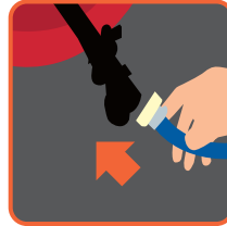
RECONNECT coupling with filter washer
